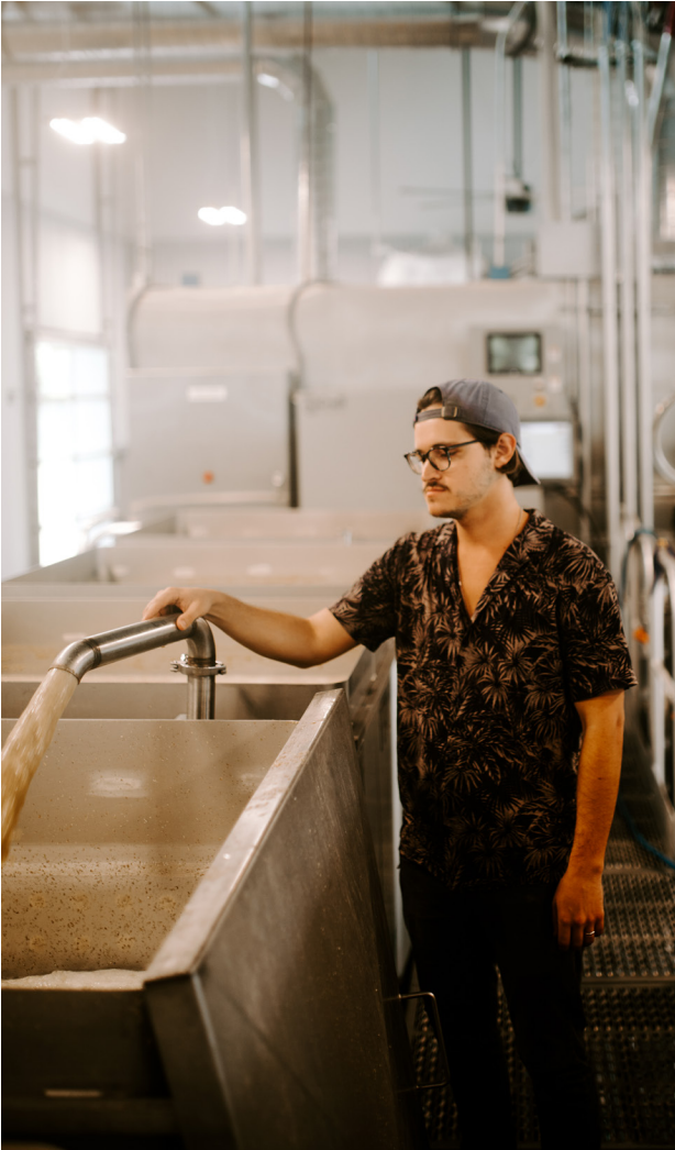
Distiller Cole Miller transferring bourbon mash from the cooker to the fermenter.
