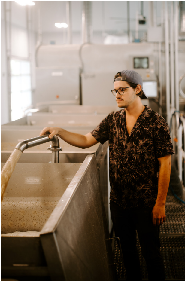
Co-Head Distiller Cole Miller transferring bourbon mash from the cooker to the fermenter.
